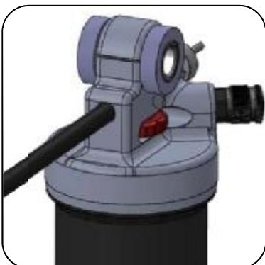
3. Use the hex wrench to turn clockwise direction and tighten
